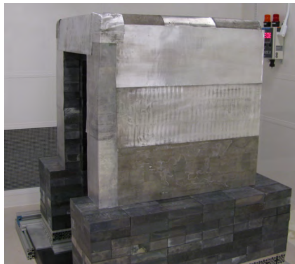
FIGURE 3.18. Lead shield wrapped in a thin layer of cadmium
