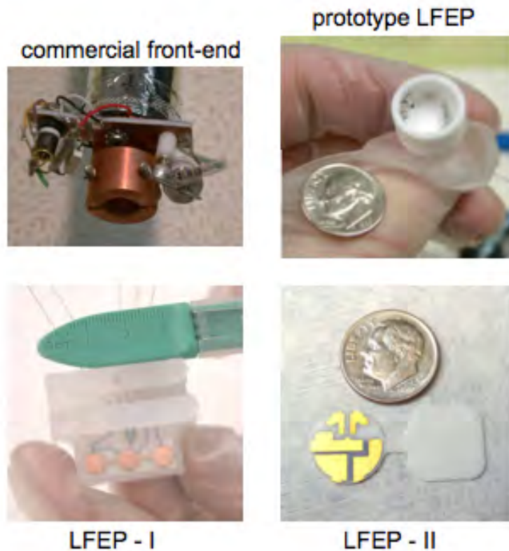
FIGURE 3.10. Evolution of LFEPs from commercial units to LFEP-II for Cascades [49]
