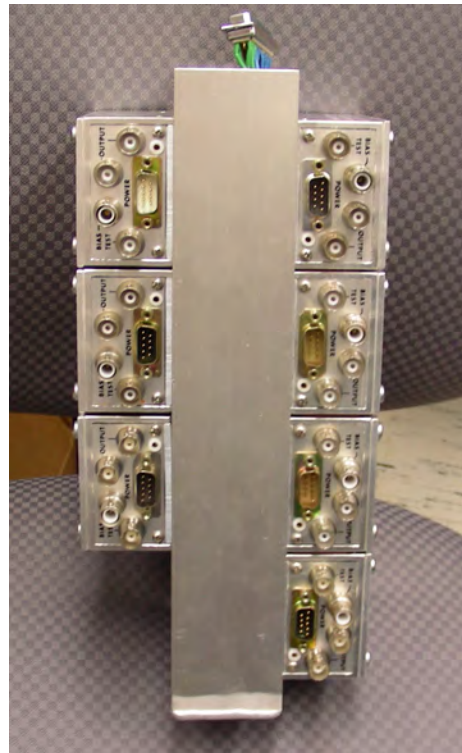
FIGURE 3.14. Close-up of a RG11B/C preamplifier
