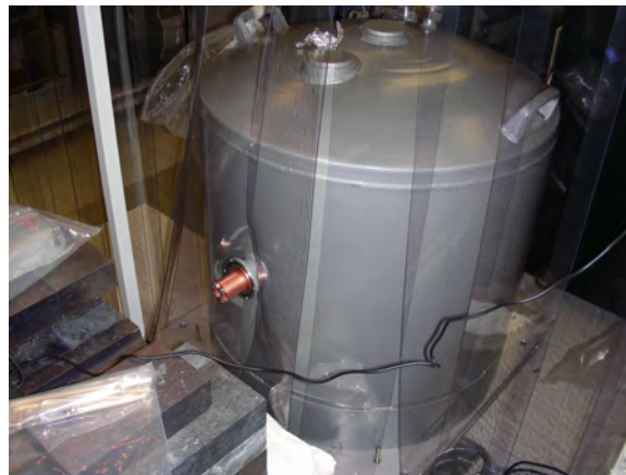
FIGURE 3.8. The liquid nitrogen dewar of Cascades prior to being attached to the lower cryostat with a thermal connection
